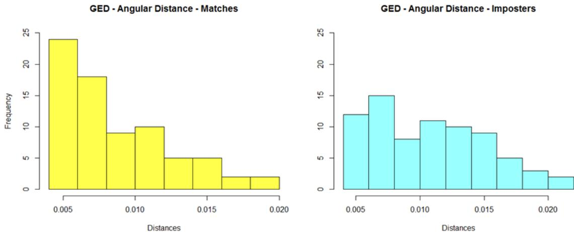
Figure 5: Histogram plots of the distance scores obtained using the graph edit distance and the vector angular distance. Prototype set size 200.
