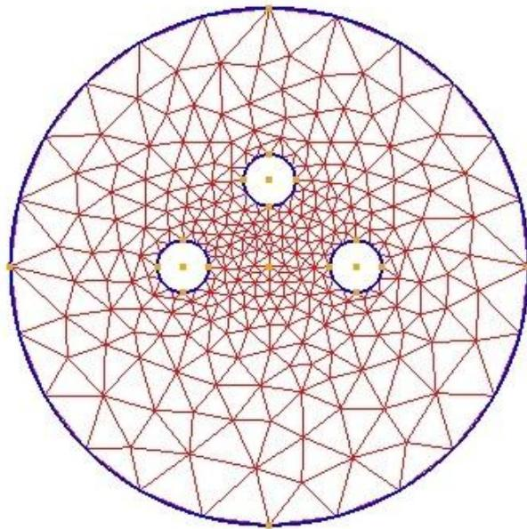
Fig 1. An example of the domain over which the numerical calculations were performed as well as a typical mesh of the domain.
