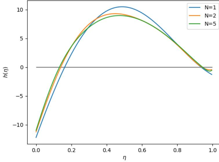
Figure 5: Graph of  $h(\eta)$ , using  $\bar{\alpha}_{2n,R}$  given by (37). Parameters given by (27), with  $D = 0.548$ . Note one large unstable ice cap, one small stable ice cap, stable snowball earth state and unstable ice-free state.
